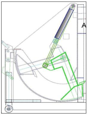
Using a scoop action compaction ram, the self-cleaning cylinders and all associated parts are housed in the top of the machine, away from any waste. This means there is no inspection hatch, no filth, no stench, no routine operator cleaning (that never gets done!), no expensive breakdowns, no replaced hoses (all common problems occurring over time with standard "straight push" portable compactors, see pics below) and thankfully no more hassle.
