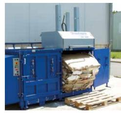
The hydraulical bale ejector for an easy and safe bale ejection.
