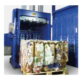
Hydraulical bale ejection
